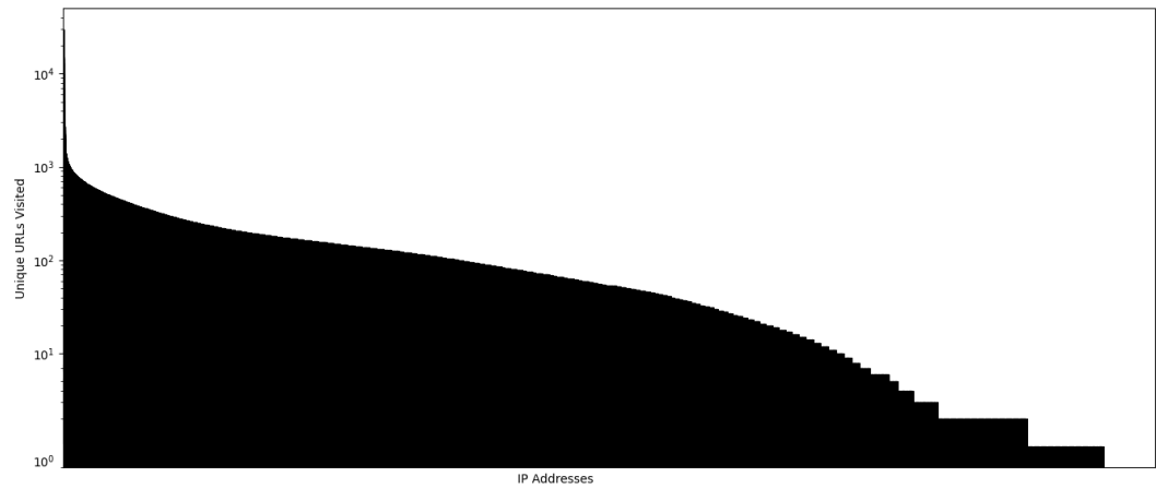
Figure 5.6: Distribution of hosts based on unique URLs contacted. The X-axis represents the hosts, while the Y-axis shows the count of unique URLs each host connected to, displayed on a logarithmic scale in decreasing order.
